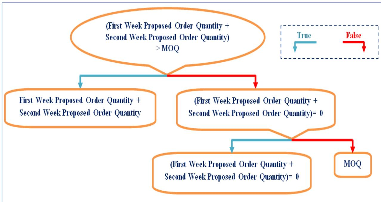
**Fig. 5 Release Order Quantity Model for Class A and B**
